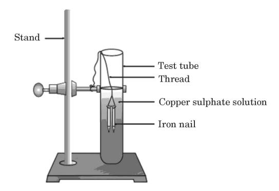
Study the experimental set-up shown in the diagram and write chemical equation for the chemical reaction involved. Name and define the type of reaction. List two other metals which can be used in place of iron to show the same type of reaction with copper sulphate solution.
